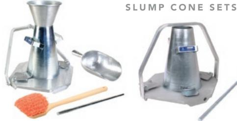
Slump Cone Test Set— H-3635 For measuring slump of freshly mixed concrete. Set includes: H-3636 Base Plate, H-3638 Funnel, H-3639.20 Brush, H-3640 Slump Cone (standard steel), H-3651 Tamping Rod w/ 6" scale on handle, H-3731 Scoop. Shipping wt. 25 lbs. (11.3kg).
