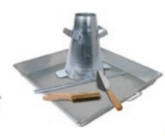
Slump Test Set— H-3645 Set includes: H-3640 Slump Cone (standard steel), H-3800 Brush, H-3650 Tamping (Puddling) Rod, H-3725 Cement Immersion Pan, H-3760 Trowel. Shipping wt. 24 lbs. (10.9kg)
