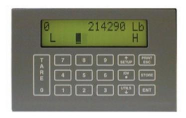
For hard-copy test documentation, up to 750 tests can be stored in memory and printed directly on an optional serial-port printer or transferred to a PC through an RS-232 serial port. The print function allows the operator to print only the current test or all stored tests at once.
