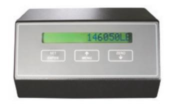
$\pm .5\%$  of indicated load from 1% to 100% of machine capacity, exceeding ASTM C-39 and E-4 requirements.
