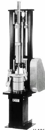
4" and 6" compactors can be easily converted for testing either 4" or 6" samples by ordering the desired size hammer and mold separately.
